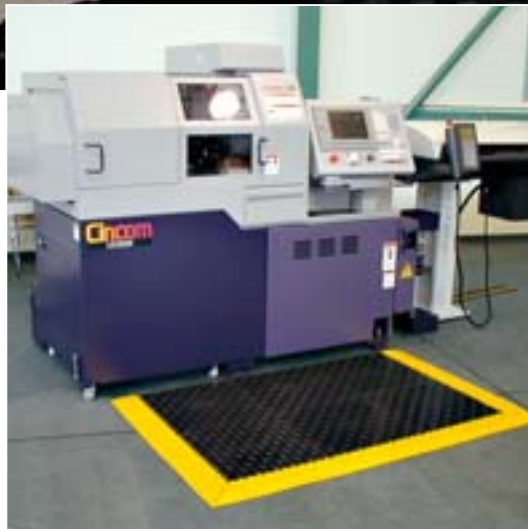
1 Large Machinery Chequerplate is used to provide an anti-fatigue anti-slip surface in front of a CNC machine. The interlocking tile system is more cost-effective than matting available in rolls as there is no wastage. The ramps that interlock with the tiles ensure that there is no trip hazard and provide an extra safety feature.
